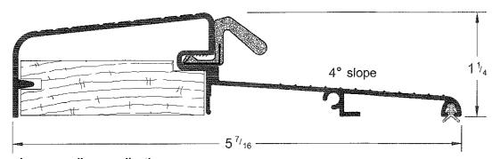
Full length insert for glue-down or nail-on applications.
